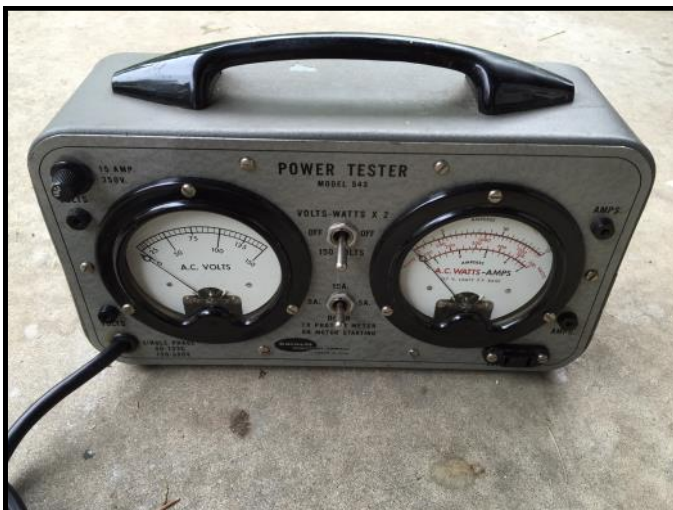
Old "power tester" device displays both line voltage and current / watts being drawn from generator.
