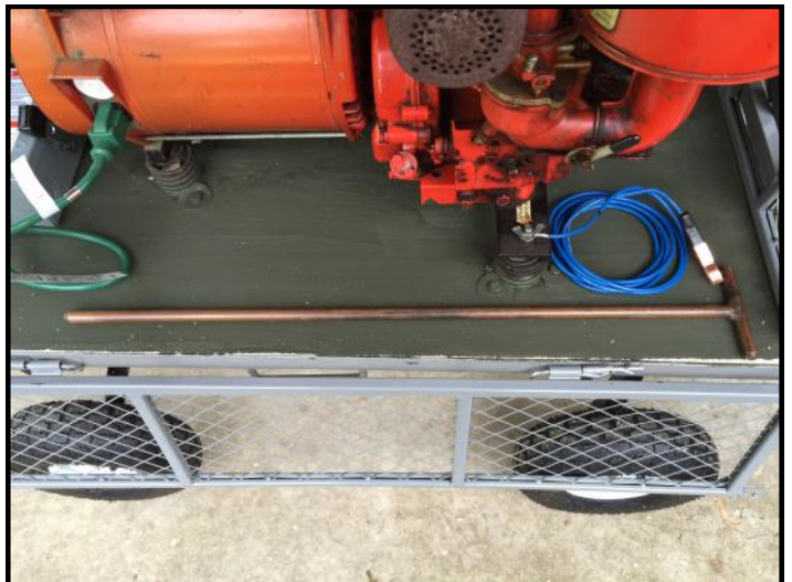
A short ground rod is often sufficient for a temporary installation. A longer ground rod may be required for sandy or rocky soil
