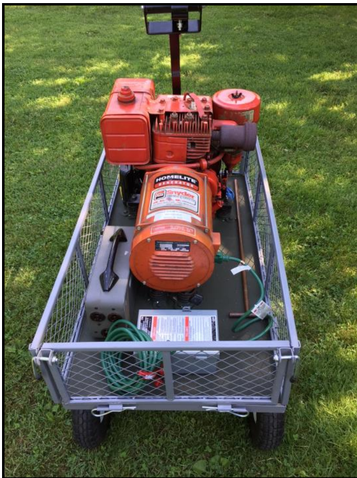
Generator mounted to garden cart. The sides fold-down for easy access for generator maintenance. The cart also works nice for transporting accessories. Note disconnect switch fused for 15-amps
